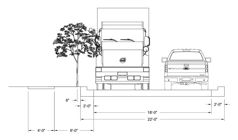
Centerline of street will shift 1 foot north to reduce impact on downhill driveways on the south side
